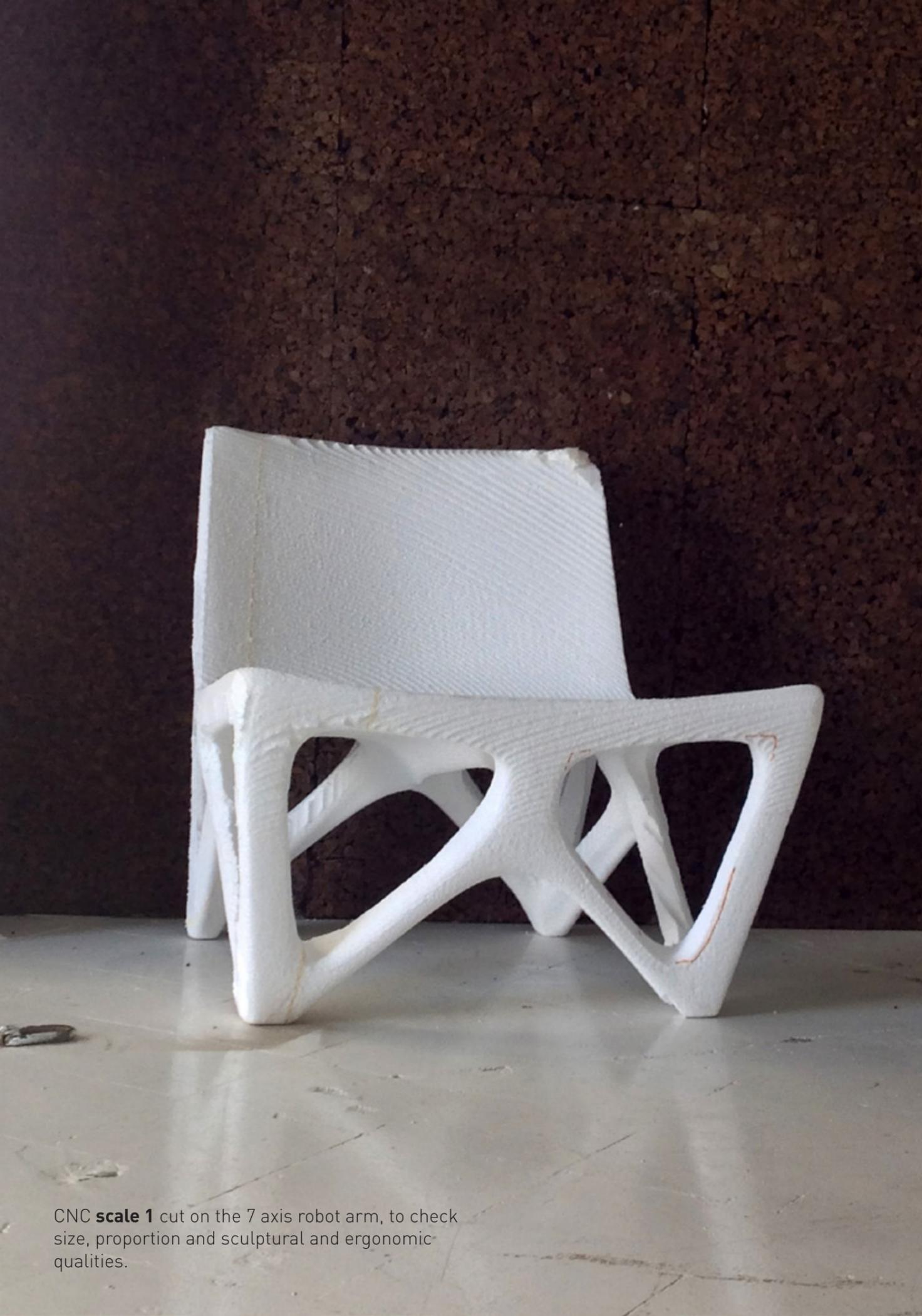
CNC **scale 1** cut on the 7 axis robot arm, to check size, proportion and sculptural and ergonomic qualities.
